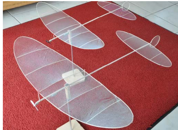
Fig. 3 Two cap models with hyperbolic wing geometry, direct drive with 3 Farad span 55 cm (4,4 g) and 45 cm (4,0 g), flight time = 2:30.
