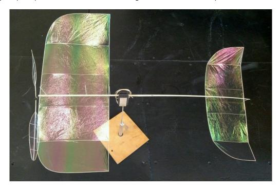
Like the modifications implemented in the previous model, I have further extended the tailboom and increased the stab area. The result is a very stable model that seems relatively oblivious to mildly choppy conditions. The require stab incidence seems "just right". On the record flight, Girder Grabber V climbed all the way to the peak of the roof in less
