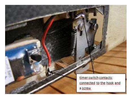
Hopefully from the above it will be seen that the timer supports both towline release from a bungee/straight tow or circle towing without any changes in timer configuration required because from a bungee or straight tow, once the glider is released there is no mechanism to further operate the microswitch which could "re-arm" the timer.
