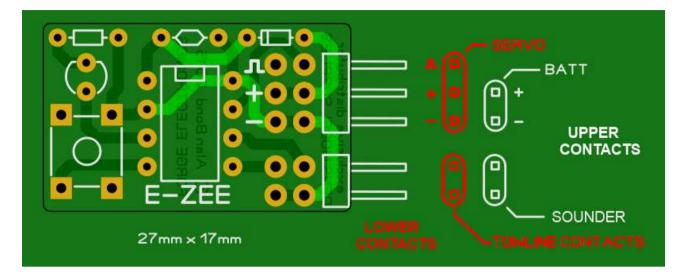
The battery lead usually coloured red/black, connects to the upper two pin header on the timer as shown in the image above and the D/T servo to the lower three pin header. Note the polarities of the battery and servo leads. The piezo sounder and towline contacts connect to the upper and lower two pin headers respectively and are not polarity sensitive.
