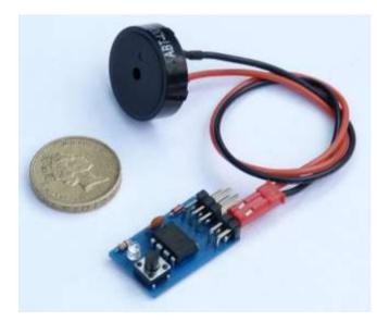
The supplied piezo sounder is a passive device and is driven by the timer in the same way that a loudspeaker is driven by an amplifier. This is to distinguish it from some piezo "buzzers" that look similar but contain integral drive electronics – *these types will not work with this timer.*
